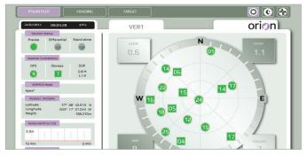
The above image is a display of a GNSS polar plot and position status information in Orion Software.
