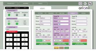
The above image displays the configuration of targets within the Orion Software.
